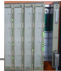
Expansion racks with digital input/output cards
