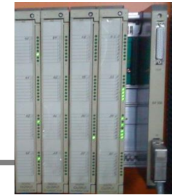
Expansion racks with digital input/output cards
